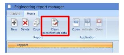
This function removes all data which are not necessary for future regeneration of the report. It does not delete e.g. embedded external pictures neither Screen shot pictures from SCIA Engineer.
