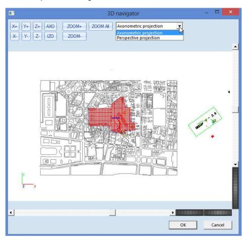
It is also possible to switch between axonometric and perspective projection.
