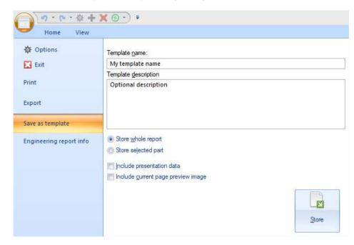
By default the report template contains only the necessary definition of report items. But it is possible to store also presentation data with the template. In such case the content of tables will be immediately visible after inserting it into a new report.
