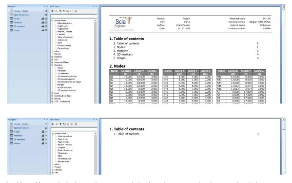
Locking of items: locked report items are excluded from the regeneration. It means that their content which is displayed in the Report preview is fixed. It can be used e.g. for comparison between result for two variants of one model or as a prevention against accidental deleting of results of time demanding checks.
