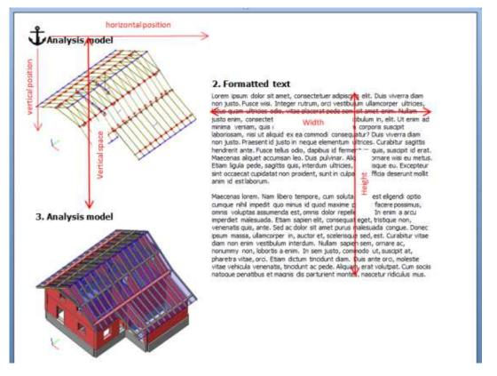
**Width** and **Height** properties are available for Formatted texts only. Width defines the maximal width of the text column. Height can define the exact height. The height is calculated automatically when the 0 value is chosen in the property window.
