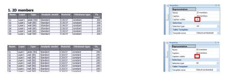
The user can reduce the content of the table by using the property Type of selection.
