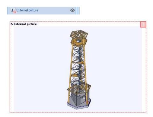
Regeneration of the picture will reread its content from the hard drive and makes its content again valid. In this way it is possible to work with external pictures in similar way as with e.g. XRefs in AutoCad.
